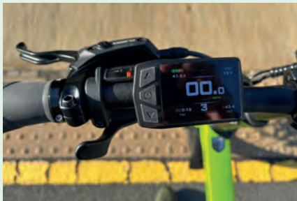
Left: Your left hand changes both gear and assistance mode, as a throttle is on the right
