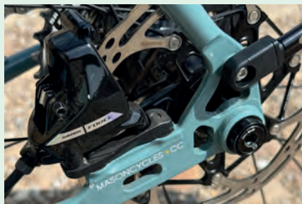
Left: With beefier dropouts, a T47 bottom bracket and larger diameter tubes, the Mason gives a stiffer ride
