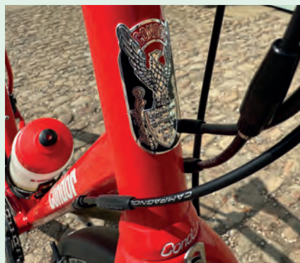
Left: The Condor Fratello is essentially a modern update of the classic clubman's bike Below: External gear cables run under the down tube and BB
