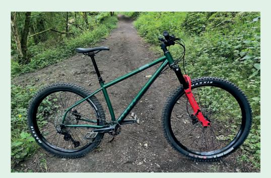
2.6in tyre in the frame and a 3in one in the fork, at least in drier weather. The rims are wide enough for 2.6in tyres.
