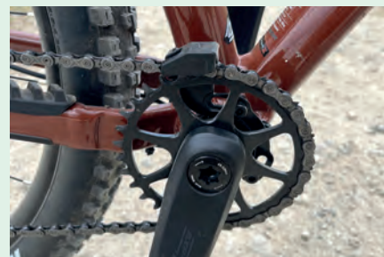
Middle: Shimano CUES is fine but it lacks the overall range and shift quality of Deore Bottom: Rowdier riders will appreciate the chain guide
