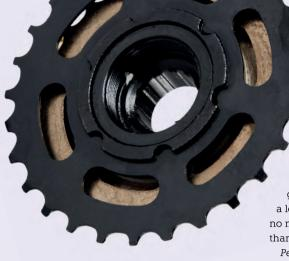
inside after use in heavy rain, the pawls may seize and refuse to engage, the springs may break and the bearings wear prematurely. There have, no doubt, been plenty of imaginative get-you-homes, such as using wire to tie the largest sprocket to the spokes, although this loses the freewheel function...
