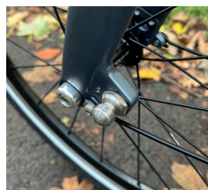
Top: The axle hook and seatpost lock the folded G Line together Bottom: The Tern's Anchor Bolt should do the same. It didn't
