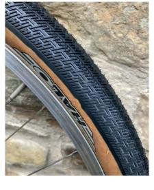
The sidewalls feel nice and supple, and this is backed up by the tyre's weight, which at 505g for the tan sidewall version is impressive given its width and the amount of tread. The black sidewall version is 20g heavier.
