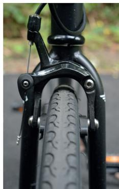
**Above:** Mid-drop sidepull brakes means room for mudguards even over these nominally 28mm wide tyres
