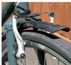
**Above:** V-brakes allow the use of a more comfortable fork than would be the case with disc brakes
