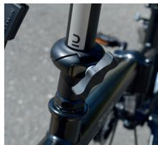
**Bottom:** The stem hinge simply clamps closed. Make sure you do this one up properly before setting off!
