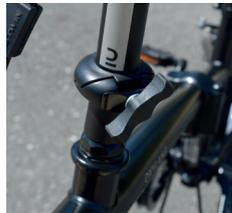
**Top:** The frame hinge won't open unless you undo the QR lever and lift the cylinder upwards against spring tension
