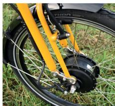
**Above:** Bafang front hub motor is fairly powerful but, with the head tube battery, makes the bike front heavy
