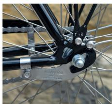
**Above:** A coaster brake provides reliable braking that doesn't wear rims or depend on grip strength.
