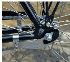
Above: A coaster brake provides reliable braking that doesn't wear rims or depend on grip strength.
