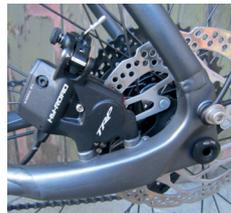
**Above:** Old-school cables operate hydraulic pistons in the bulky but effective TRP HyRd disc brake callipers
