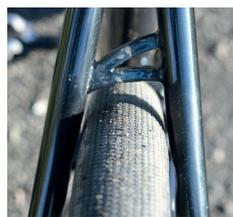
**Top:** Toe overlap with a size 42 shoe. This is awkward when steering around stuff off-road at slower speeds
