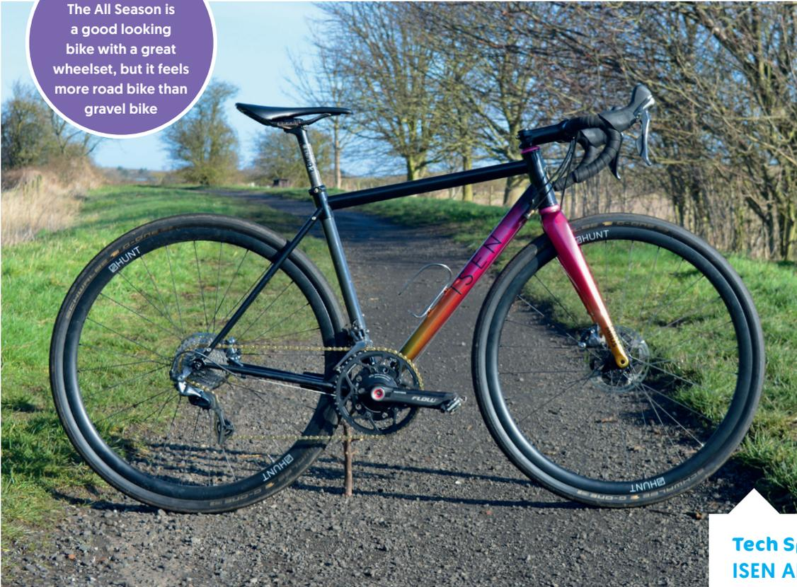
“The test bike has an ENVE carbon seat tube bonded into steel lugs, a frame-builder’s flourish that’s £449 extra
