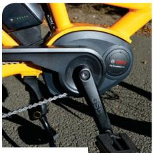
Assistance is effective at low cadences, with a max torque of 63Nm. Hill starts are easy
