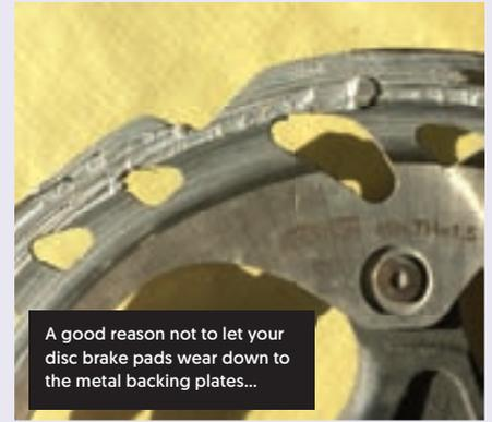
A good reason not to let your disc brake pads wear down to the metal backing plates...
