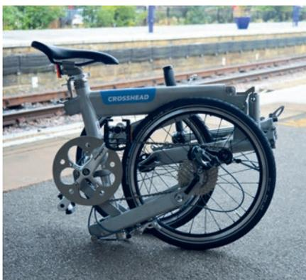
**Above:** Bigger than Brompton, slightly smaller than a Birdy, it will easily fit an end-of-carriage luggage rack
