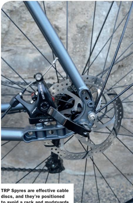
TRP Spyres are effective cable discs, and they're positioned to avoid a rack and mudguards
