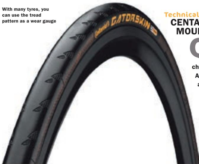
have been known to wait until the carcass fabric shows through before replacing a tyre, whether it's slick, provided with a wear indicator, or heavily treaded. This is a desperate measure and the tyre should ideally be replaced before it gets to that state. However, the last few molecules of tread rubber covering the fabric can wear through in a couple of miles, and a tyre tread that looks fine at the start of a ride may not last to the end.
