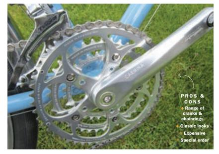
range, it should be possible to assemble a triple (or double) to suit almost any cycling activity. The test triple has 48/38/28 chainrings and 175mm cranks installed on TA's Axix Light bottom bracket axle.
