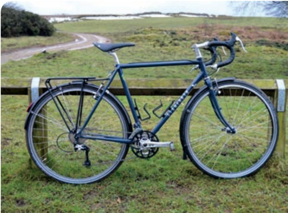
**Below:** The 48-36-26 chainset provides better touring gears than a road triple
