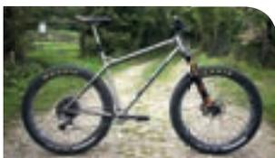
**1 Curtis AM+ £1,150+ (frame)** Fillet-brazed from a mix a tubesets, this hardtail has a longish top tube, a 66.5° head angle, and clearance for 27.5+ tyres. Takes a 120mm fork – or longer. [curtisbikes.co.uk](http://curtisbikes.co.uk)
