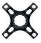
so. Only one option immediately presents itself: TA, distributed in the UK by Chicken Cycle Kit (chickencyclekit.co.uk), make a five-arm 94mm PCD double spider that will fit your existing cranks and allow you to fit a 29t or 30t inner chainring (also made by TA). RRP is £69.99.
