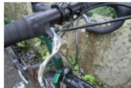
**Above:** The Dawes's auxiliary levers allow braking from the tops but preclude using a bar bag
