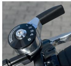
**Above:** The 5-speed drivetrain has a good range (256%) but outside of flat terrain the hub needs a larger sprocket
