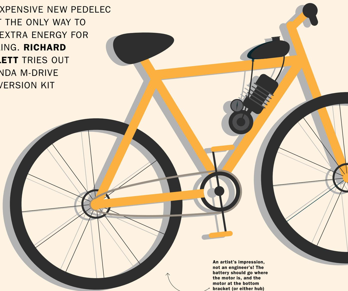
An artist's impression, not an engineer's! The battery should go where the motor is, and the motor at the bottom bracket (or either hub)
