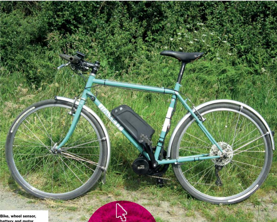
Bike, wheel sensor, battery and motor
