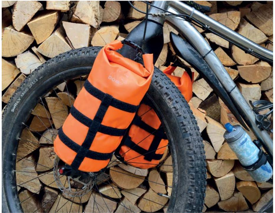
**F**REE PARABLE'S MONKII System is a way of carrying liquids and luggage via the bottle bosses. Circular cleats fix in place, sitting proud of the frame or fork, and the Monkkii stuff slots onto them. There are clamp-on mounts for bikes lacking bosses.
