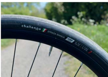
**Above:** The tyres are nominally 33mm but stretch to 39mm wide on these 19mm-internal rims
