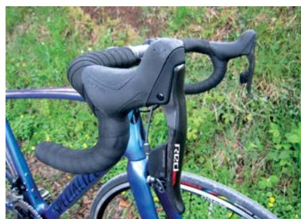
**Above:** The right shifter moves the rear derailleur to a smaller sprocket, the left moves it to a bigger one. Press both shifters together, the front mech moves up or down
