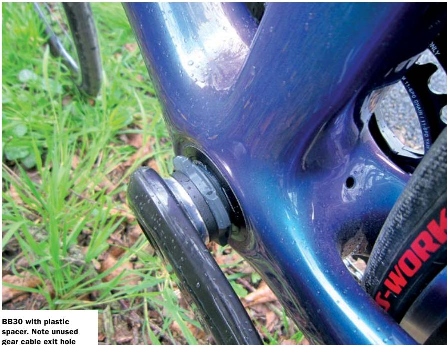
BB30 with plastic spacer. Note unused gear cable exit hole
