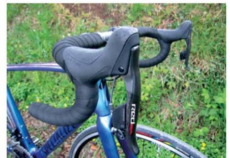
**Above:** The right shifter moves the rear derailleur to a smaller sprocket, the left moves it to a bigger one. Press both shifters together, the front mech moves up or down
