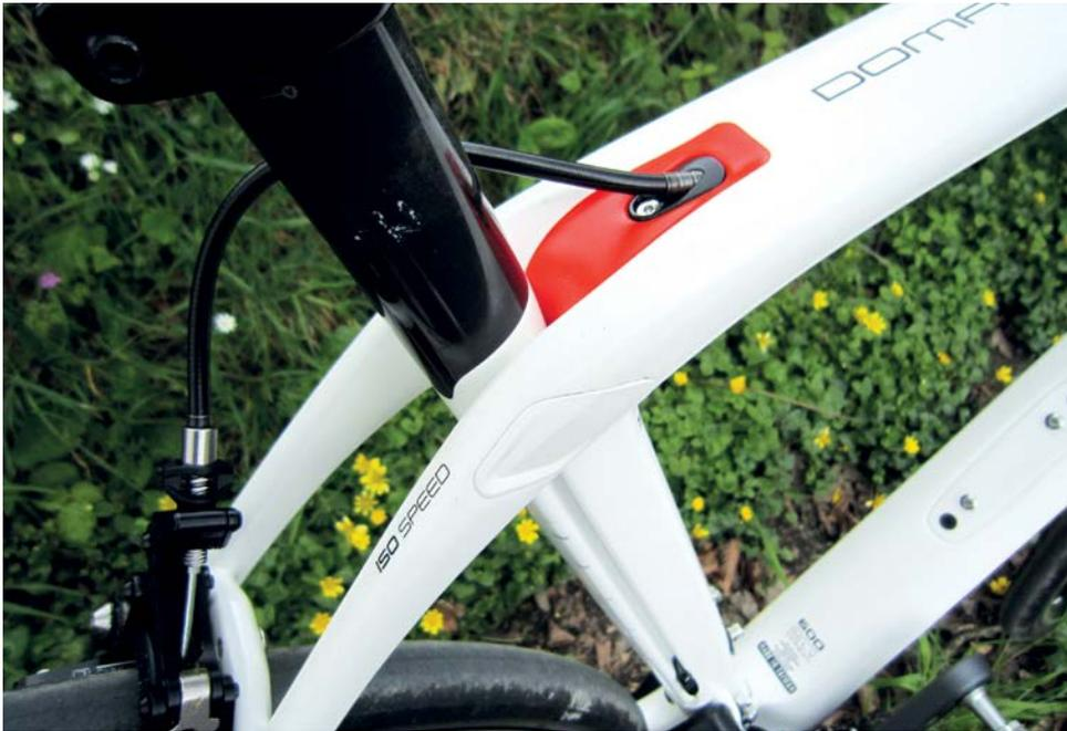
**Clockwise from left:** IsoSpeed de-coupler gives fore-aft movement. Complex callipers. Di2's shift setup is normal: RH lever = rear mech
