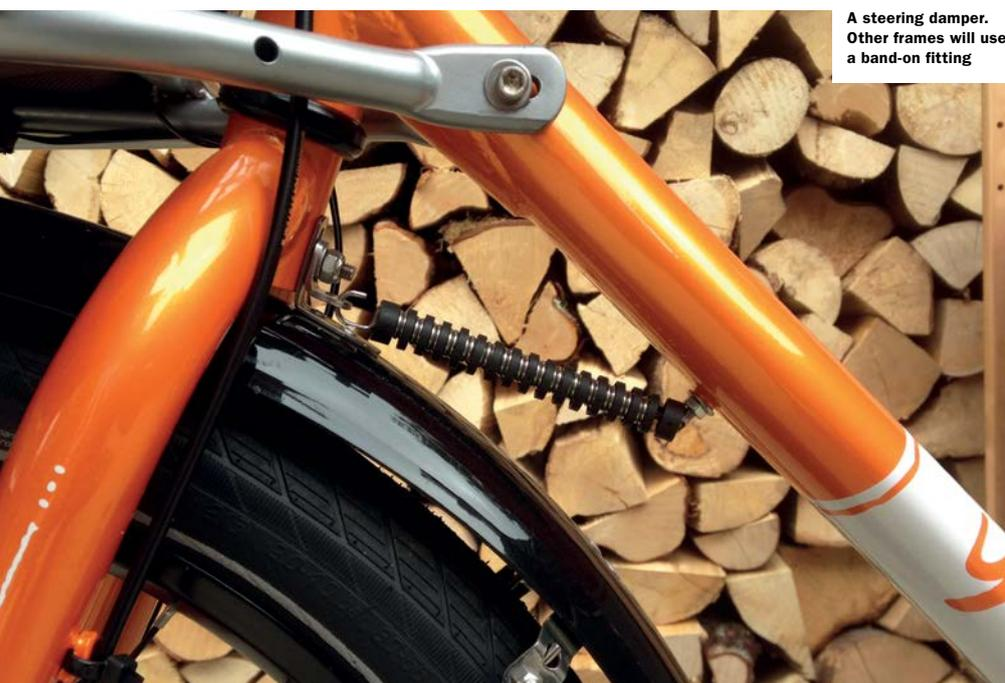
A steering damper. Other frames will use a band-on fitting
