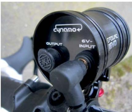
**Above:** No on-off switch means daytime running lights – unless you unplug the input cable
