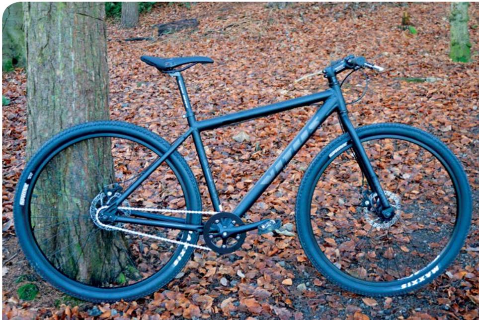
**Below:** Chain tension is via short track ends. Longer ones would simplify wheel refitting by providing more slack
