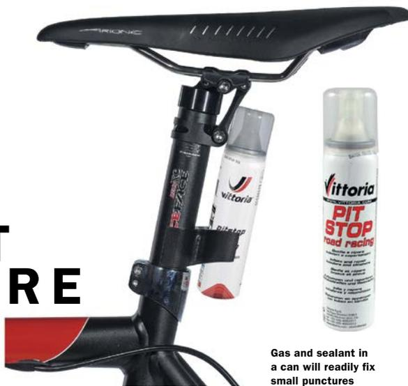
Gas and sealant in a can will readily fix small punctures
