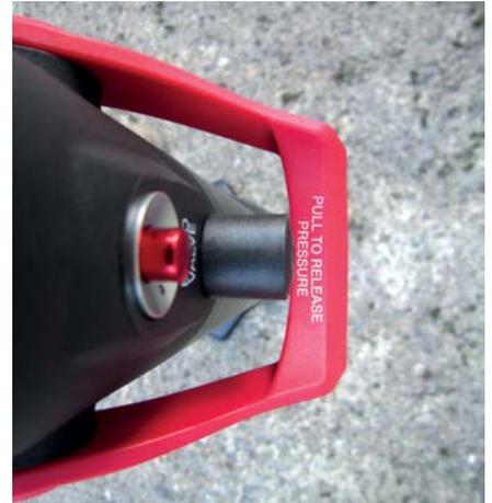
**Above:** Pulling the lever releases a large volume of air quickly in order to seat tubeless tyres
