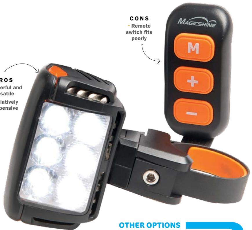
light. There are six high-power LEDs in the lamp, in two rows of three. The bottom row shines through a diffuser in the lens, giving a flood effect, while the top three are unfiltered and provide a strong central spot. Available lighting modes are: top row only, bottom row only, or both rows. I wanted depth *and* width off-road so used both rows all the time.
