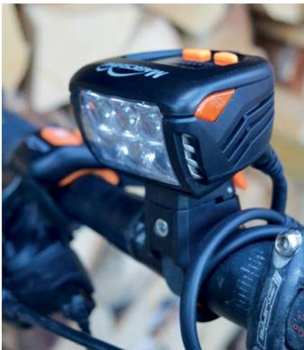
**Above:** The quick-release bracket is secure but sits the lamp quite high, so it could be vulnerable in a fall
