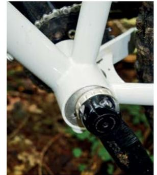
■ This 100mm-wide eccentric bottom bracket was made specially for Singular. It's a good solution for accommodating different diameter wheels
