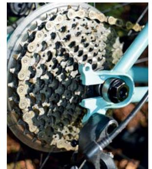
■ The Wednesday does it with rear-facing dropouts. With different wheels/tyres, bottom bracket height can't be fine-tuned but the wheelbase can be
