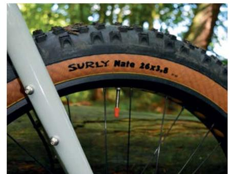
**Above:** Both bikes come with 26×3.8in tyres but you can fit bigger – up to 26×4.6 or more in both frames and fork. Alternatively, 29+ wheels and tyres will fit
