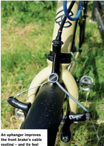
An uphanger improves the front brake's cable routing – and its feel
