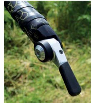
■ Bar-end shifters are simpler and probably more durable, and this Microshift rear one can be switched to friction operation if the indexing goes out of whack
