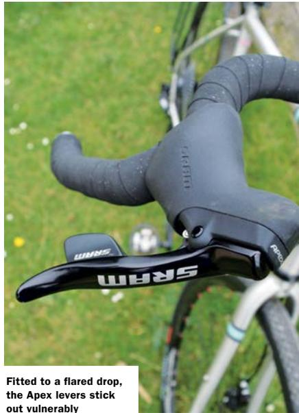
Fitted to a flared drop, the Apex levers stick out vulnerably
