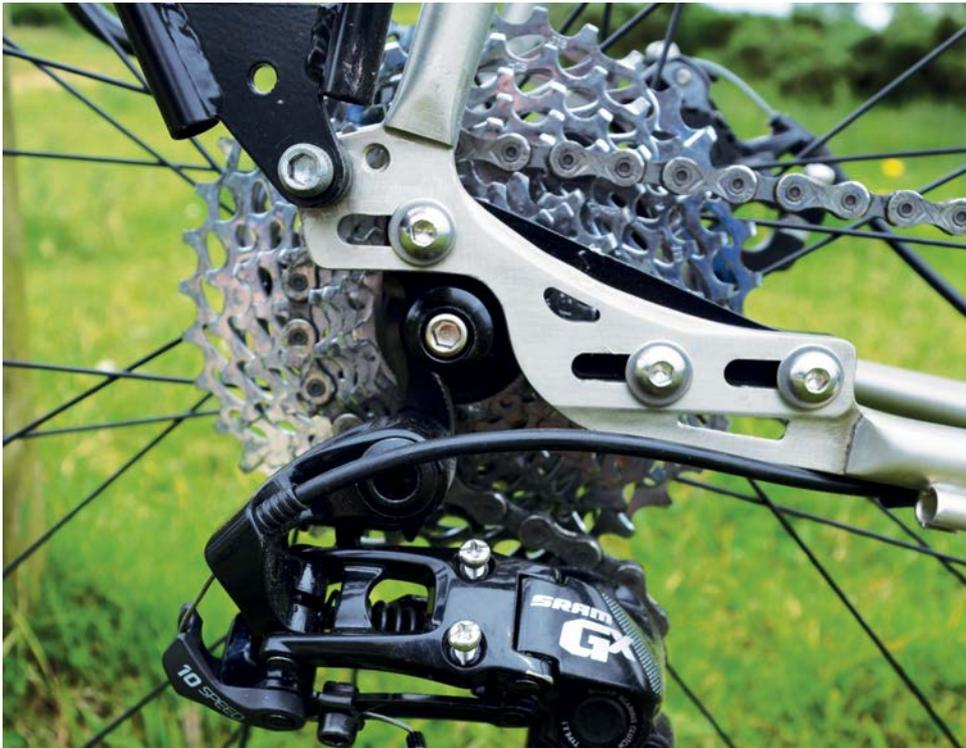
**Left:** The Darwin's dropouts allow up to about 15mm of fore-aft movement. So the frame is hub gear and singlespeed compatible. The lower rack eyelets use stronger M6 bolts (which the borrowed Tubus rack accommodates)
