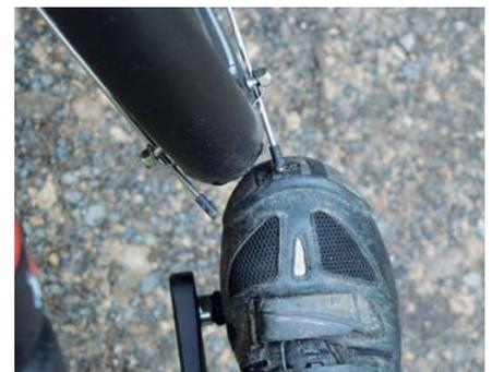
**Above:** Toe overlap is more troublesome on a bike like the HoBootleg, which will often be used for slow-speed meandering, than it is for a fast-riding road bike
