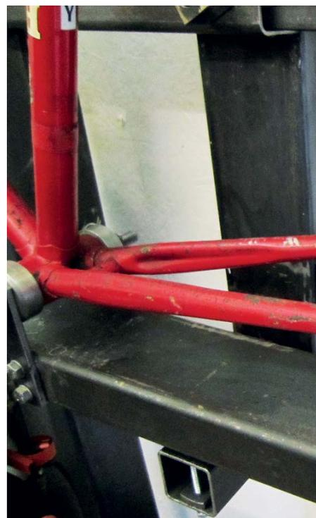
source of a crack, and a visible crack as terminal unless you know of a skilled aluminium welder. Similar considerations apply to early carbon-fibre frames: check carefully that structural integrity has not been compromised.
