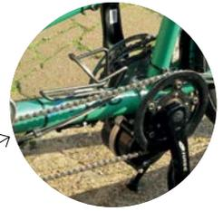
The Sunstar bottom bracket motor provides assistance for up to 80km per charge
