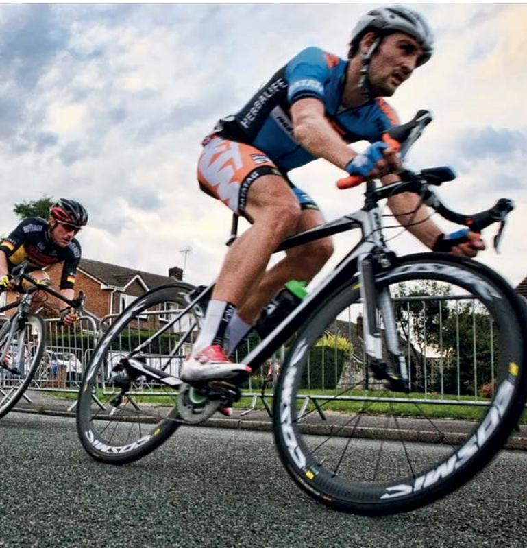
This is a big difference, so why does rolling resistance not worry racing cyclists? At racing speeds, it contributes a very small part of the overall drag affecting the rider. At 45kph (28mph), aerodynamic drag makes up around 85% of the total and small differences between tyres make a negligible difference to speed. Races can be won by fractions of a second, so it is still worth having fast-rolling tyres... But their effectiveness is easily overlooked at racing speeds.
