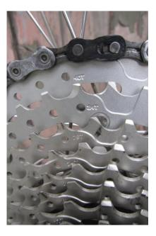
very small chainring. This is a good idea: bigger sprocket combinations tend to wear the chain more slowly, and there's less likelihood of breaking the chain - the smaller the ring, the greater the chain tension for a given force applied at the pedal. This is also why small chainrings can give a 'spongy' feel to the transmission.
