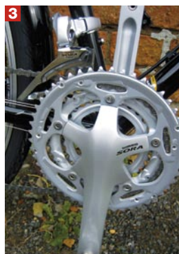
3 A road triple: the 39-tooth middle ring is okay, if less useful than a 36, but the 30T inner and 50T outer are too big for a loaded tourer
