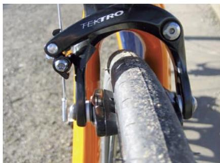
● 57mm brakes mean plenty of room for mudguards above 25mm tyres. Without guards, 28mm tyres would fit
