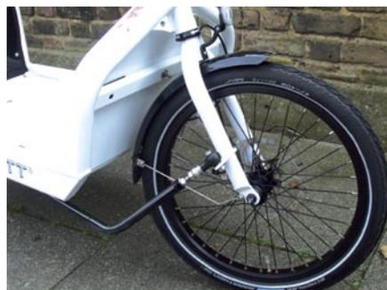
● (Above) The Bullitt's front load platform is easy to keep an eye on. Steering is via a rod to the fork
