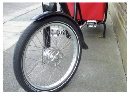
● (Above) The 8Freight's hubs are supported on one side only. Puncture repairs are easy, upgrades less so
