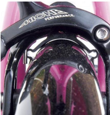
● (Above) Good clearance under the brake calliper is wasted by thick mudguard fittings
