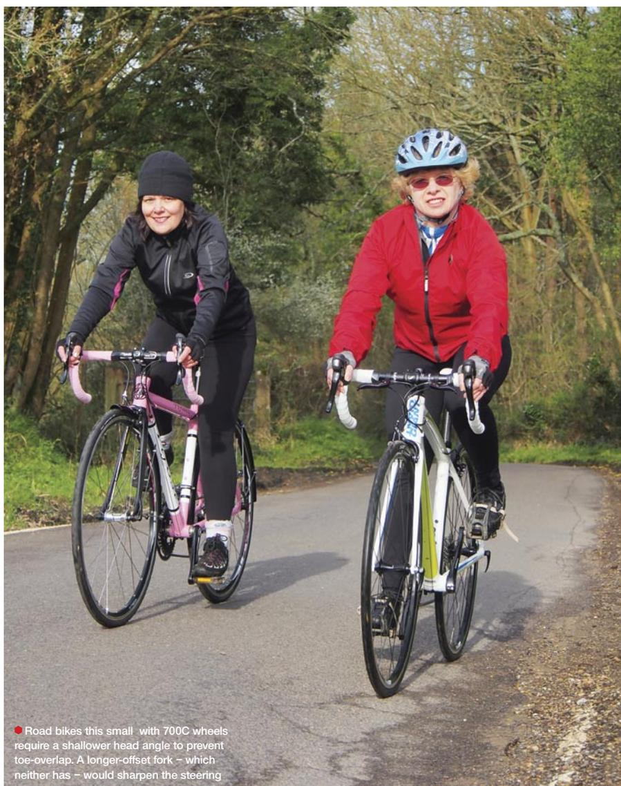
● Road bikes this small with 700C wheels require a shallower head angle to prevent toe-overlap. A longer-offset fork – which neither has – would sharpen the steering
