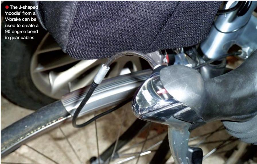
• The J-shaped 'noodle' from a V-brake can be used to create a 90 degree bend in gear cables
