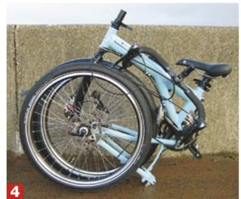
There are no hinges as such; the non-suspended rear triangle pivots underneath and other parts detach. To begin, you telescope the upper seat post into the lower post. Then you remove the front wheel.
