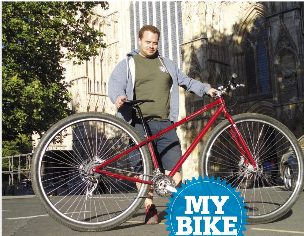
(Left) Dylan with his prototype, which fits riders from 5ft 3in to 6ft 5in. Production versions are custom built for the rider. They won't fit riders smaller than that but can, of course, be designed for taller riders (Below) The prototype uses 48-hole tandem hubs laced to 36in rims designed for unicyclists
