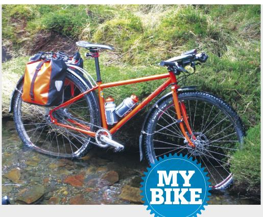
(Left and below) Isla's bike with its 11-speed Alfine hub. She says: You don't get any lower bottom gears than with the 8-speed. So I run it with the biggest sprocket that I can fit on, which is a 23. And I've got a 32 chainring to get the gears as low as I can. That's been fine for off-road touring.
