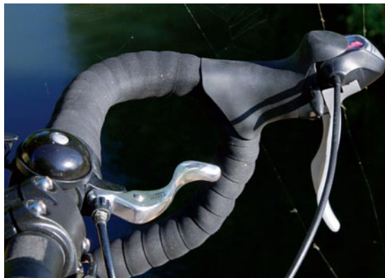
(Top to bottom) The Revolution's extra brake levers come with barrel adjusters. The Raleigh has plenty of space for the closer chainline it needs. The Raleigh's asymmetric brake straddle is stabilised by the front mudguard
